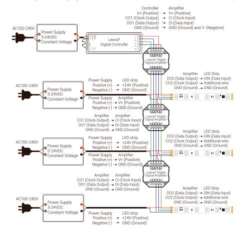
\*NOTE: The wire colors may differ from manufacturer to manufacturer, please refer to the actual solder pad pinout on the LED strip light you are using.
