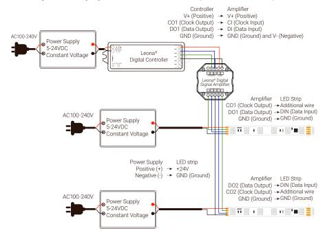
\*NOTE: The wire colors may differ from manufacturer to manufacturer, please refer to the actual solder pad pinout on the LED strip light you are using.
